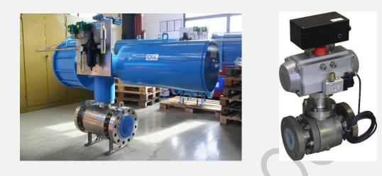
Pneumatic actuators are normally used for small and middle-sized valves, where the required torque is not so high. They are used when there is a requirement of high operation speed and when a failsafe function in emergency or when the air supply fails.
