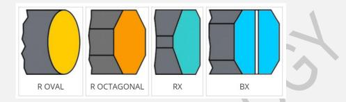
The RX type is suitable for pressures up to 700 bar. RTJ is capable of sealing itself. The outer sealing surfaces make the first contact with the flanges. A higher system pressure causes a higher surface pressure. Type RX is interchangeable with the standard R-models.
